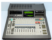
Yamaha DMR-8 (1990) integrated digital mixer and tape-based digital multitrack recorder
