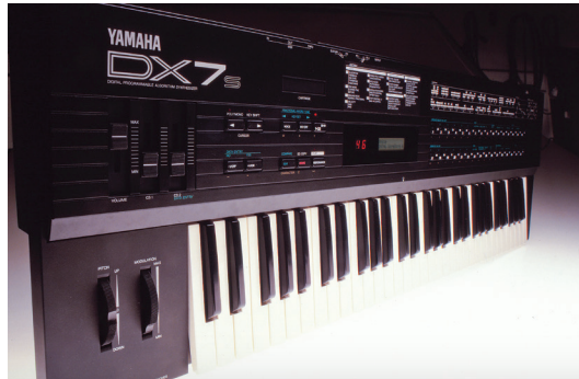
Yamaha DX7 (1983) a new palette of synth sounds via frequency modulation
