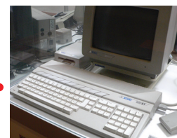
Atari ST (1985) the first computer with a built-in MIDI interface
