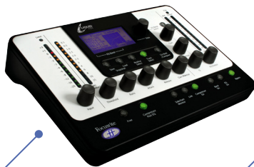
Focusrite Liquid Mix (2006) convolution-based computer add-on for hosting compressor and equaliser plug-ins
