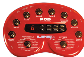
Line 6 Pod (1998) guitar-amp and speaker modelling hardware
