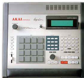
Akai MPC60 (1988) MIDI sequencing and sampling hardware with performance pads — designed in conjunction with Roger Linn
